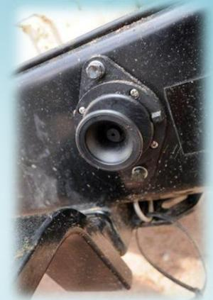
Also available is an additional male connector and 200mm lead, for fitment to an additional trailer. Early in 2011 EZ Connector expects to have a 14-pin version and a two-pin, 100-amp-capacity connector set to replace Anderson-type connectors. The two-pin model is currently being validated by the US Army.
