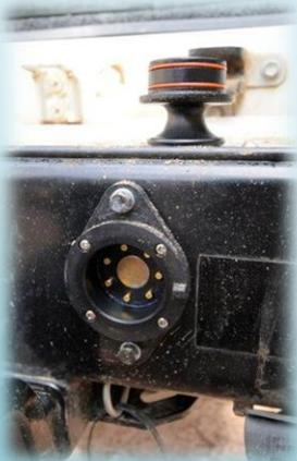
The female (vehicle) side has seven recessed, spring-loaded brass pins that press against seven brass contacts in the male section. A dummy plug and socket are provided for clean connector stowage when vehicle and trailer aren't coupled, but the latest product release is a pair of connector halves with hinged closing pieces.
